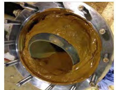
*Eroded and Corroded Ball Valve*
