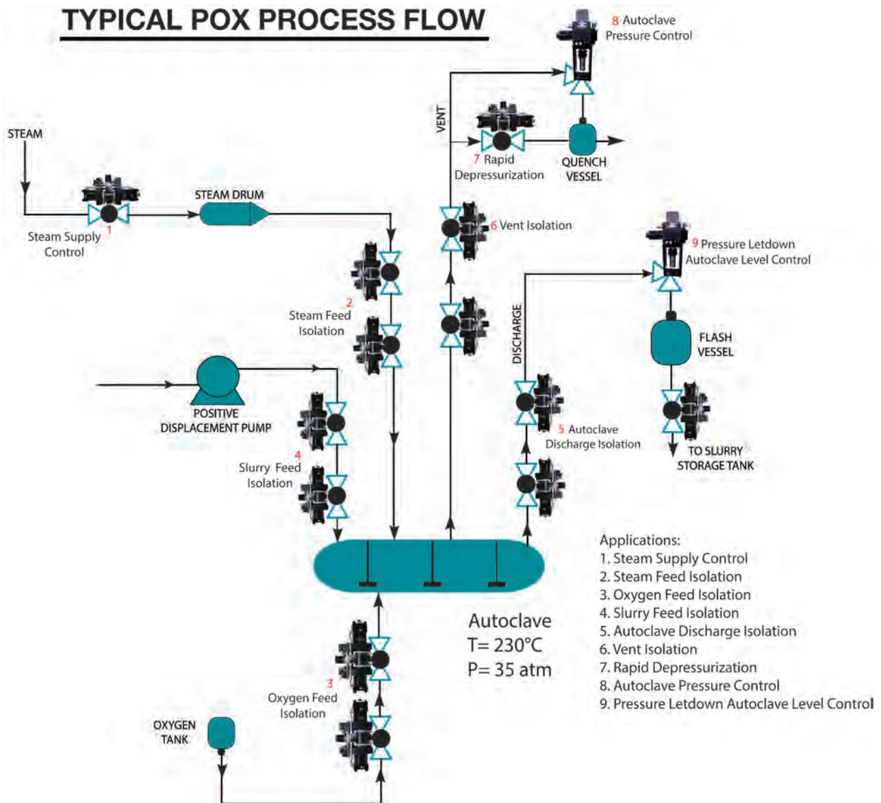
improved block valve positioning reliability were necessary and REXA's solution was self-contained [X3 MEGApac Rotary Actuators](#) based on the company's [Electraulic® Technology](#).
