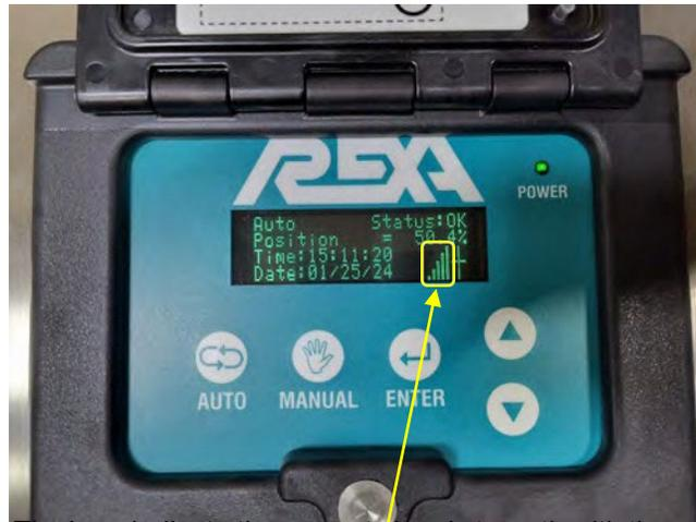
The bars indicate the current signal strength with the connected device.
