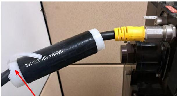
The loose end of the plastic spiral must face toward the bottom (cable) end
