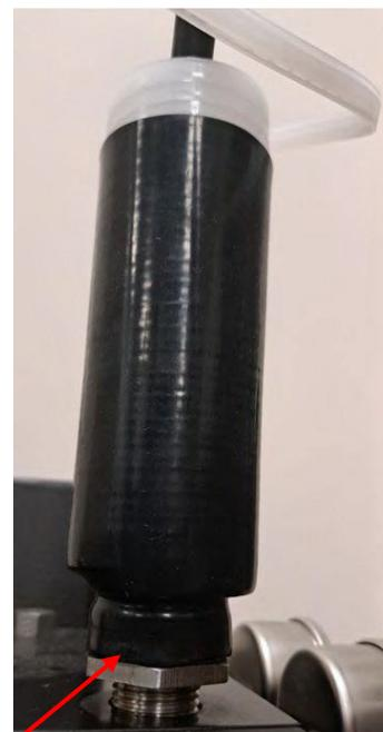
Tubing starting position must be tightly up against the large hex nut feature of the receptacle.
