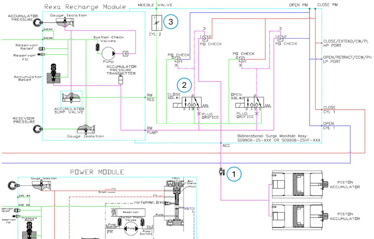
1. If manual operation of the system is required, close off Ball Valve (Item 1). This is to prevent oil backflow into the Accumulator Bottle when operating the manual override.
