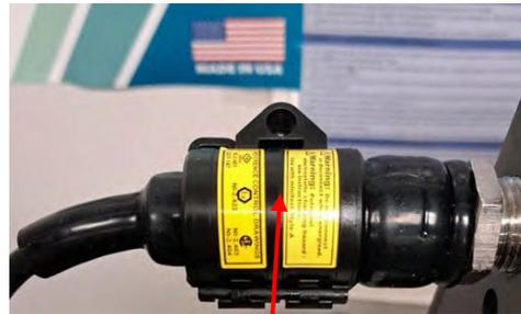
Position the LockFast over the shrink as shown and click closed. Push and twist the LockFast up the body of the shrink until it is tightly in place.
