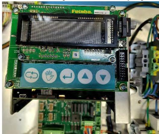
3. Use a small pair of pliers to remove the suitcase jumper located at the top corner of the board.
