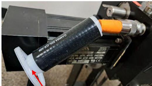
The loose end of the plastic spiral must face toward the bottom (cable) end
