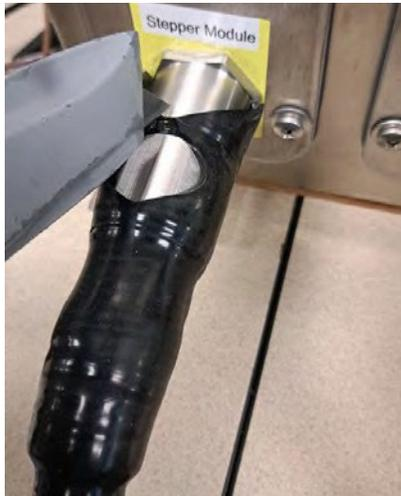
**Figure 5B – Continue scoring all the way down to cable jacket to completely remove shrink**
