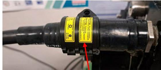
Position the LockFast over the shrink as shown and click closed. Push and twist the LockFast up the body of the shrink until it is tightly in place.
