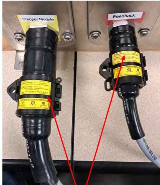
**Position the LockFast over the shrink as shown and click closed. Push and twist the LockFast up the body of the shrink until it is tightly in place.**
