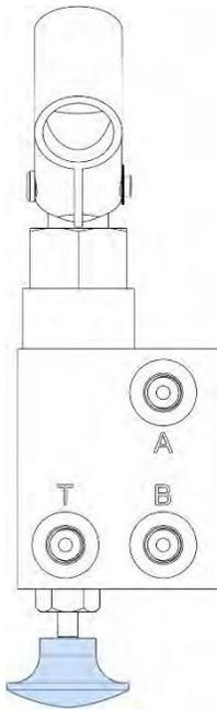
The manual hydraulic pump can be installed on all units and needs only the cylinder side of the hydraulic circuit and the Flow Match Valve (FMV) check valves to be in working order.
