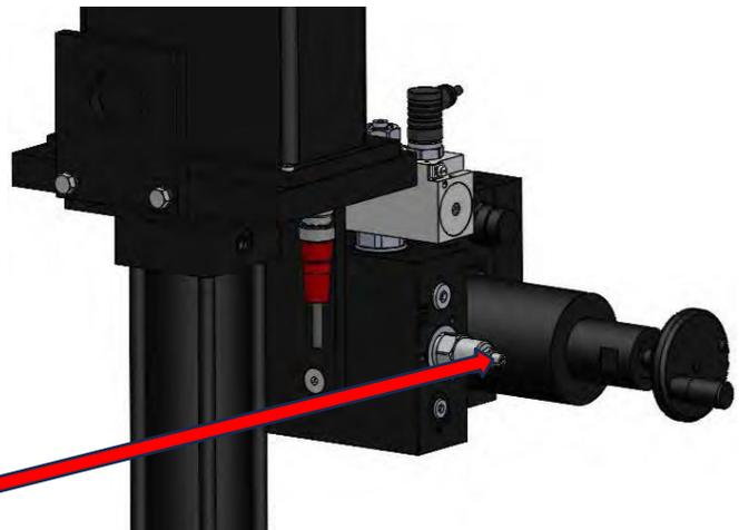
Figure 4: Needle Valve Adjustment Screw Locator
