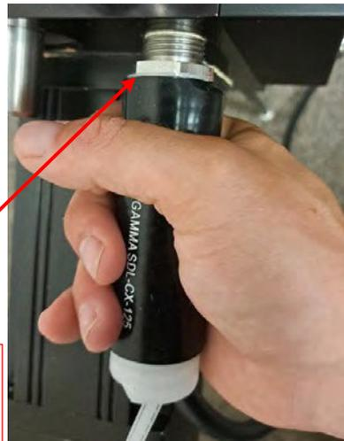
Tubing starting position must be tightly up against the large hex nut feature of the receptacle.
