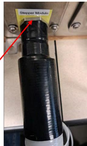
Figure 4C – Tubing after shrinking
