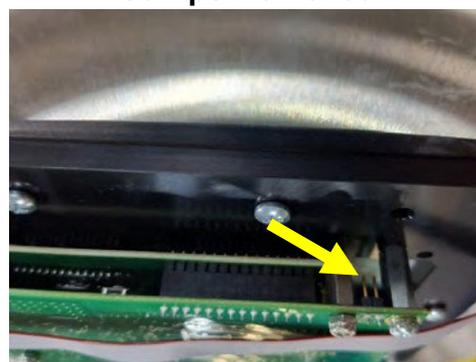
*NOTE: Use caution during removal to not drop the jumper onto any of the board assemblies and potentially cause an electrical short.*
