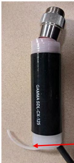
Tubing starting position must be tightly up against the large hex nut feature of the receptacle.
