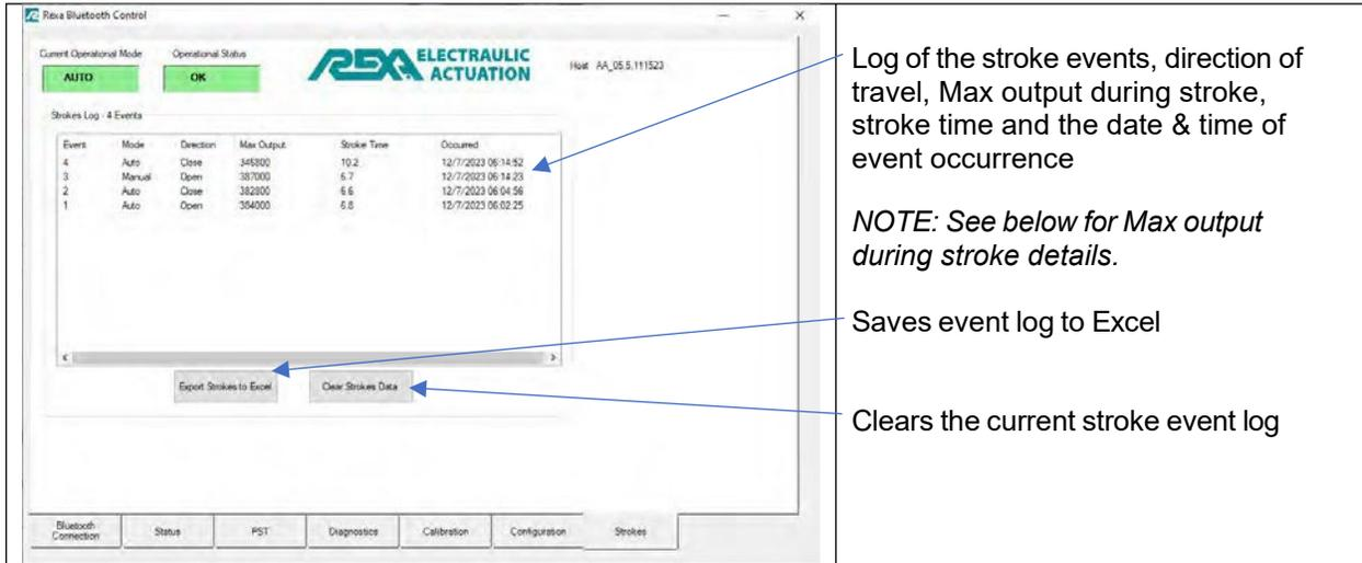
Log of the stroke events, direction of travel, Max output during stroke, stroke time and the date & time of event occurrence
