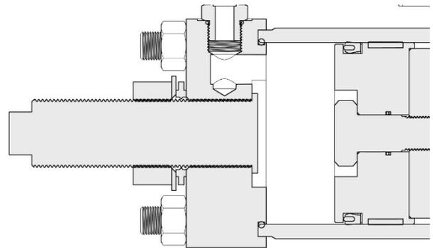
Figure 36C: 50,000 in-lbs. and Up Stroke Adjuster
