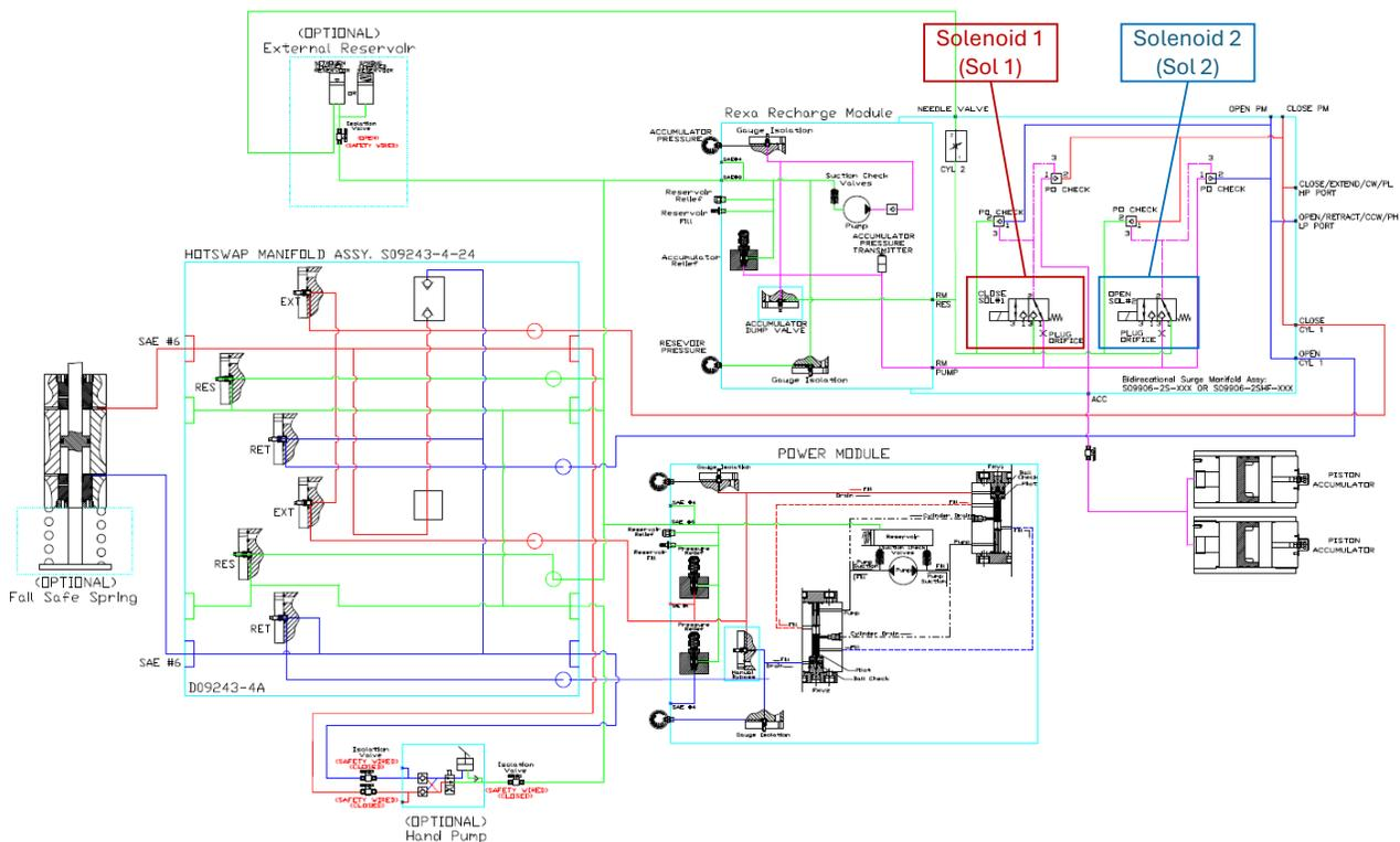
**Sol 1** is energized, and **Sol 2** is de-energized during normal operation. Upon loss of power, **Sol 1** de-energizes to fail-safe the system to the Extend/PL/CW direction. **Sol 2** is de-energized during normal operation and on loss of power; therefore, the PO checks remain closed, allowing no flow to move the actuator to the Retract/PH/CCW direction.
