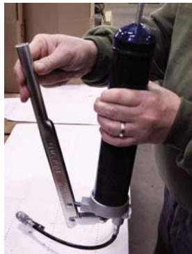
Figure 1.6.4-4 Purge the air.
