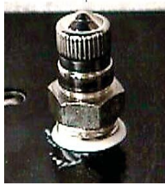
Figure 1.6.4-2 Fill Valve with cover.
