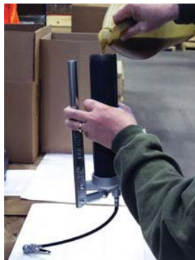
Figure 1.6.4-3 Fill the oil gun.
