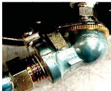
Figure 1.6.4-6 Fill Valve with Schrader fitting.
