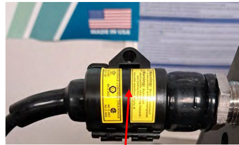
Figure 3D – LockFast secured (Small)
