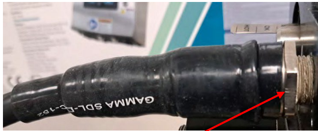
Figure 2B – Large Tubing after shrinking
