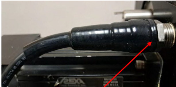
Figure 3C – Small Tubing after shrinking
