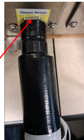
Figure 4B – Tubing Position as shrinking begins
