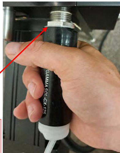
Figure 3B – Small Tubing Position as shrinking begins
