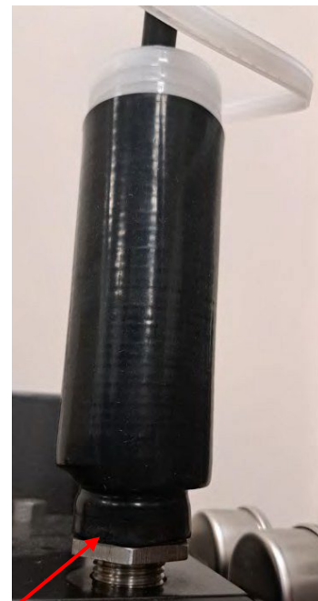
Figure 2A – Large Tubing Position as shrinking begins
