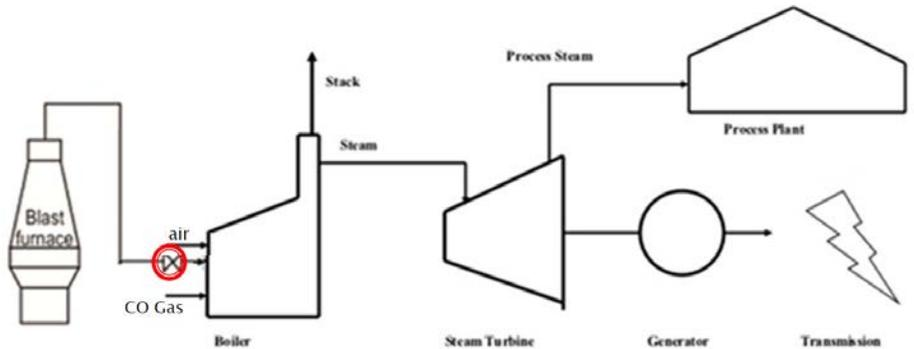
**KEY TO SUCCESS** in producing high quality steam is to have minimal process variation of incoming BFG entering the boiler. Tightly controlled pressure and gas flow rates can enable efficient combustion and boiler product steam pressure. This will in turn lead to steam with stable pressure, which is critical for efficient turbine operation and advances the plant to be utilized by product gases to produce steam and energy.
