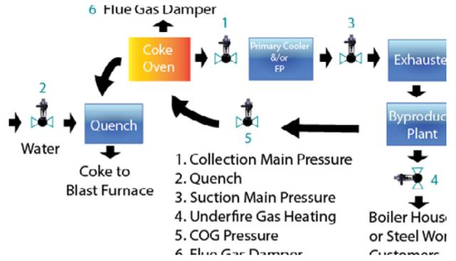
REXA Rotary or Drive Actuators have the precision (0.05%) and capability to precisely control the coke oven collection line gas pressure.
