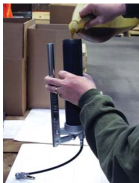
Figure 1.6.4-3 Fill the oil gun.
