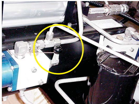
Figure C.4-1 Solenoid Manual Override Levers (Position A)
