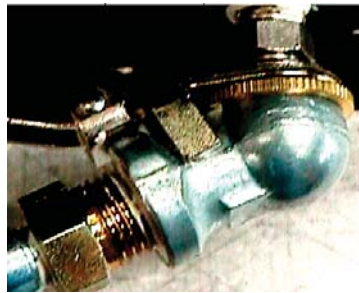
Figure 1.6.4-6 Fill Valve with Schrader fitting.
