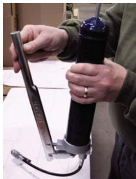
Figure 1.6.4-4 Purge the air.
