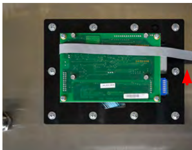
4.E.14-3 Ribbon Cable Position
