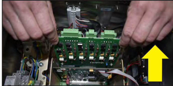
Figures 4.E.5.1-4 Contact Input Board Unseating
