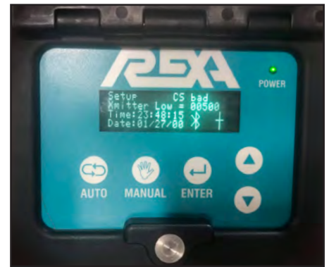
Photo 3.13.4-4 Xmitter Lo Readout
